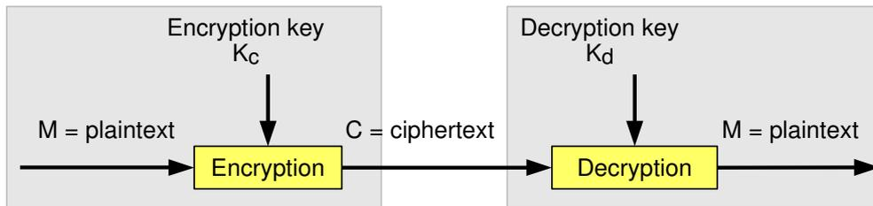
Figure 2: Overall operation of an encryption algorithm
